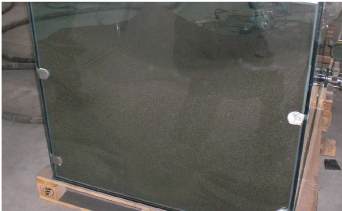
Pic 4 500mm thick 0.4MPa pressure particle movement traces
